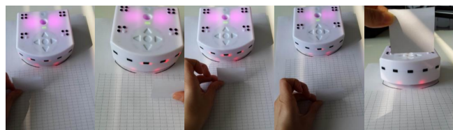
Fig. 3. Example of exercise in the semi-guided exploration activity for which student explore the intensity of the IR signal reflected according to the distance of the sensor with regard to a white piece of paper.
